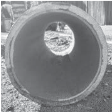
Figure 2 –replacement Cement-Lined Ductile Iron Pipe
