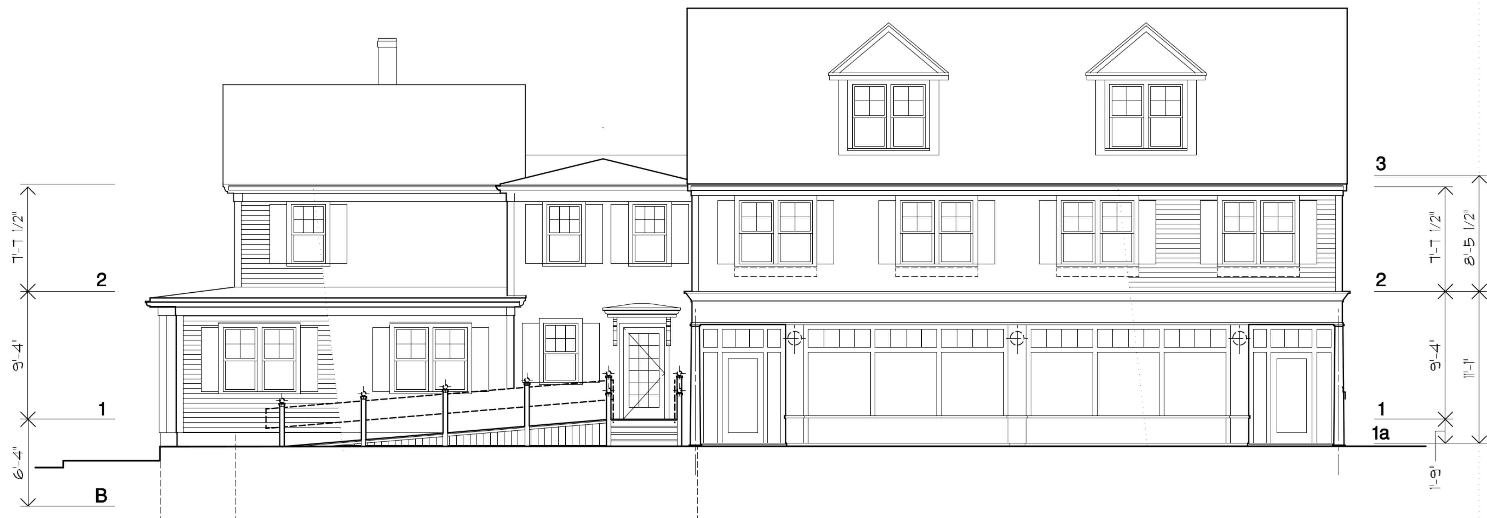
1 Front Elevation (Atlantic Avenue) - Scheme #1, 1/4" = 1'-0"
