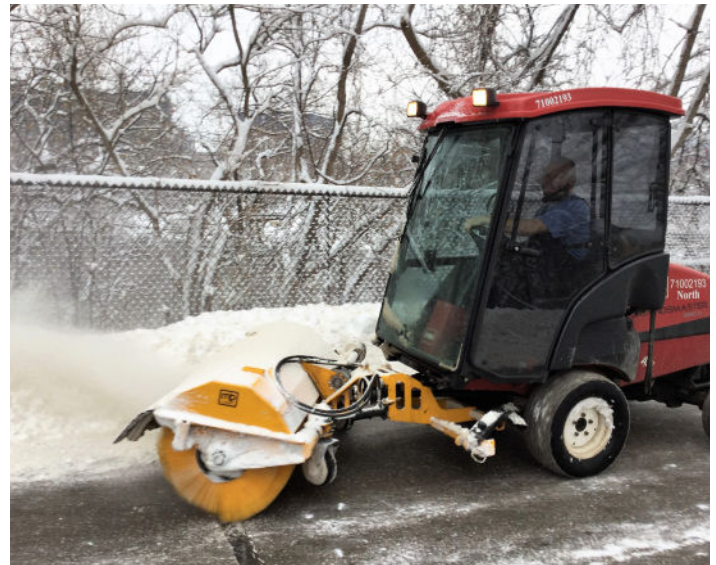
Lawn mower tractor (converted to winter maintenance vehicle) with broom
