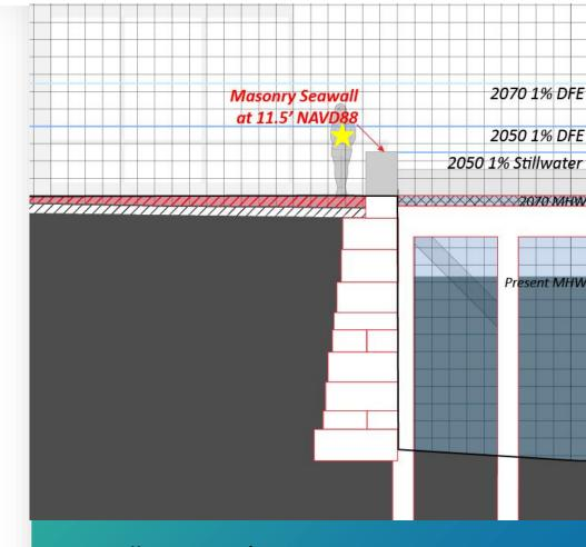
Seawall cap: 11.5' NAVD88 (could be designed to be extended in the future)
