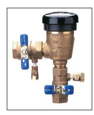
A Pressure Vacuum Breaker (PVB) device is an atmospheric vacuum breaker that can be utilized under constant pressure and that can be tested in line. These units are available in several configurations and sizes and have broad use for residential irrigation systems. Installation of these devices must be at least 6 to 12 inches higher than the existing outlet.
