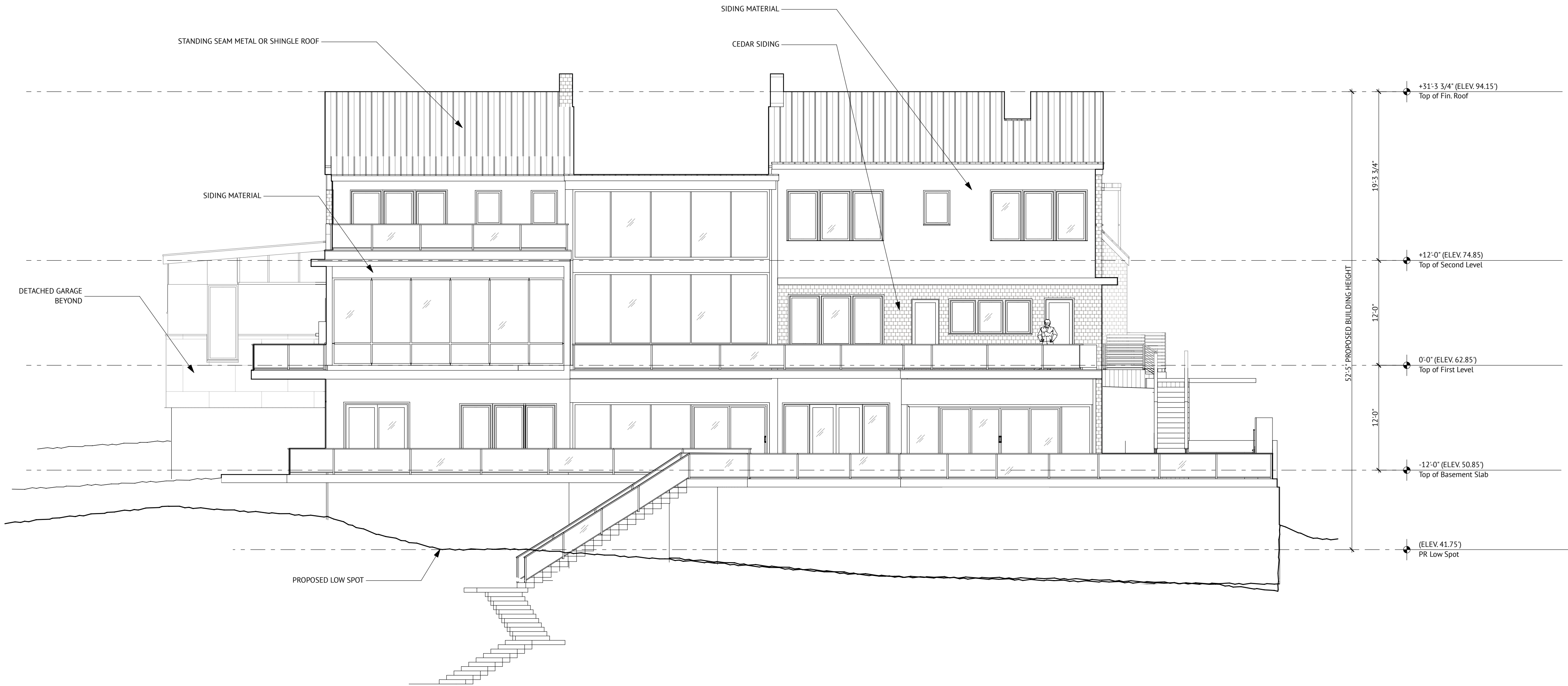
1 Proposed East Elevation SCALE: 1/8" = 1'-0"
