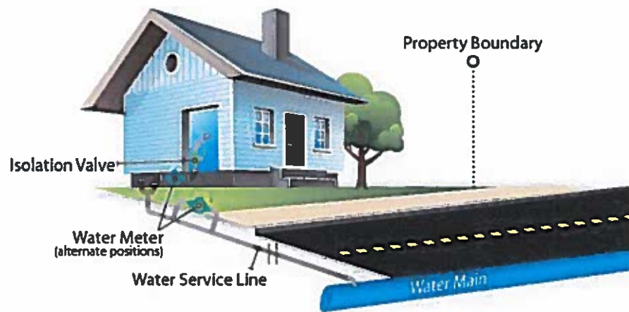
Typical location of a residential water service line (1)
