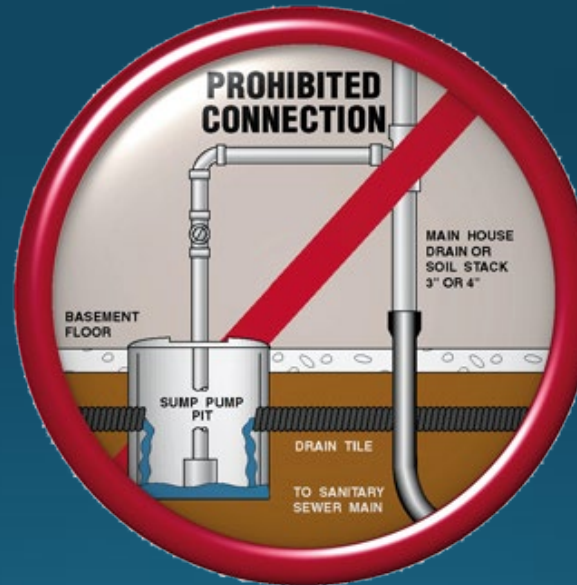
Prohibited Connection Example: Sump Pump and Downspouts connected to sewer system
